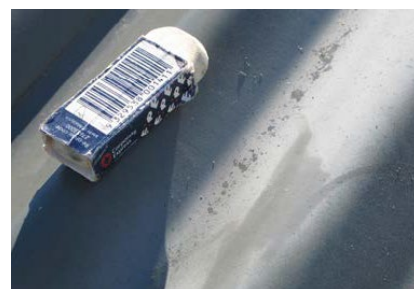
Figure 2. Rubber eraser showing colour of original painted surface beneath a removed surface layer of faded appearance
